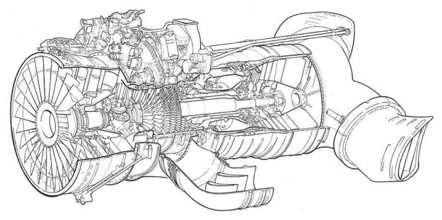
Fig. 18-2 Lift/Propulsion engine.
