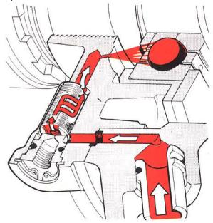
Fig. 8-11 A thread-type oil filter.
