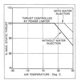
Fig. 17-1 Turbo-jet thrust restoration.
