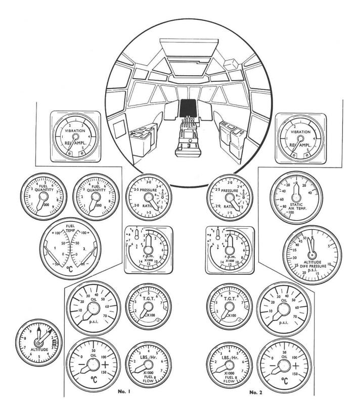
Fig. 12-1 Pilot's instrument panel - turbo-jet engines.
