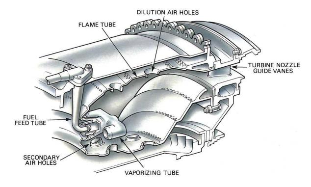
Fig. 4-5 A vaporizer combustion chamber.
