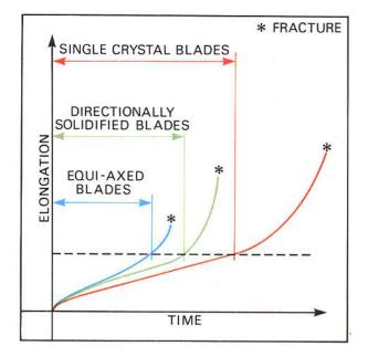
Fig. 5-13 Comparison of turbine blade life properties.
