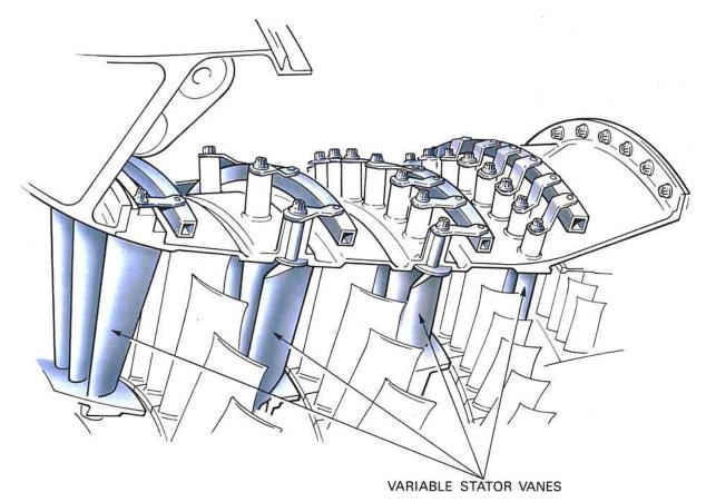
Fig. 3-15 Typical variable stator vanes.
