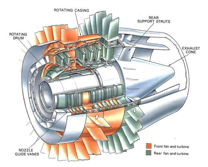
Fig. 5-10 Free power contra-rotating turbine.
