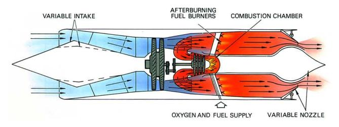
Fig. 1-12 A turbo-rocket engine.
