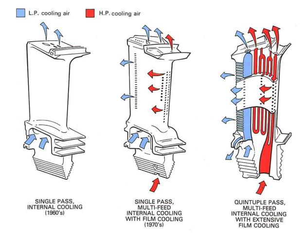
Fig. 9-3 Development of high pressure turbine blade cooling.
