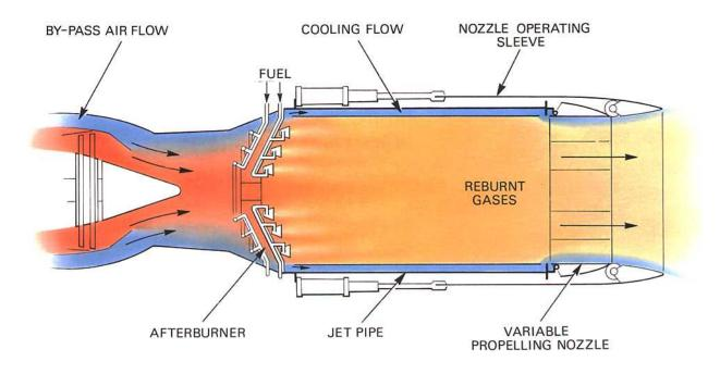
Fig. 16-1 Principle of afterburning
