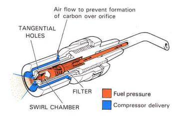
Fig. 10-16 A Simplex fuel spray nozzle.
