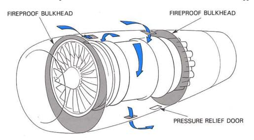
Fig. 14-1 A typical cooling and ventilation system.
