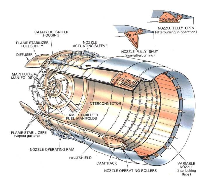
Fig. 16-4 Typical afterburning jet pipe equipment.
