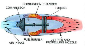
Fig. 1-2 A Whittle-type turbo-jet engine.
