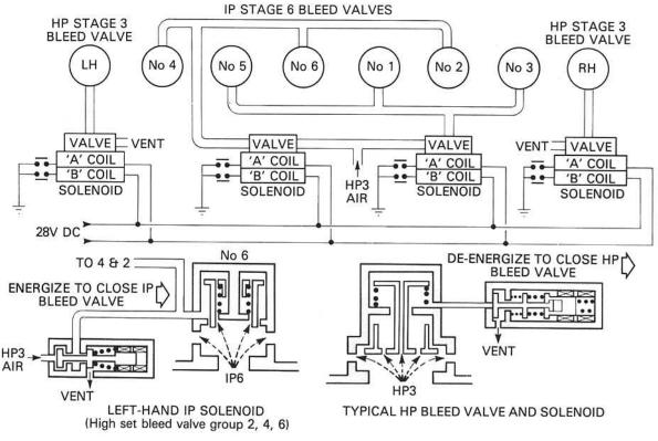
Fig. 3-18 An electronically operated bleed valve system.
