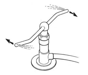
Fig. 1-5 A garden sprinkler rotated by the reaction of the water jets.
