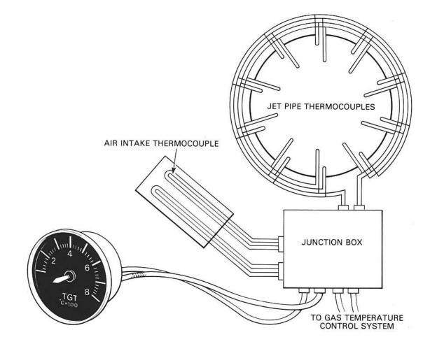
Fig. 12-8 A typical double element thermocouple system.
