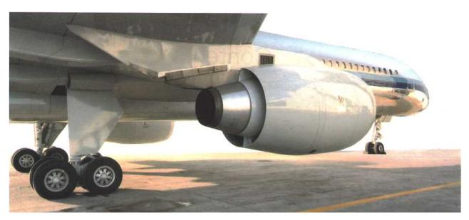
Fig. 23-1 Wing-mounted pod installation.
