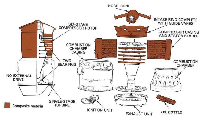
Fig. 18-10 A lift-jet engine.
