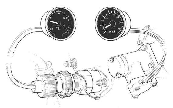
Fig. 12-9 Oil temperature and pressure transmitters and indicators.
