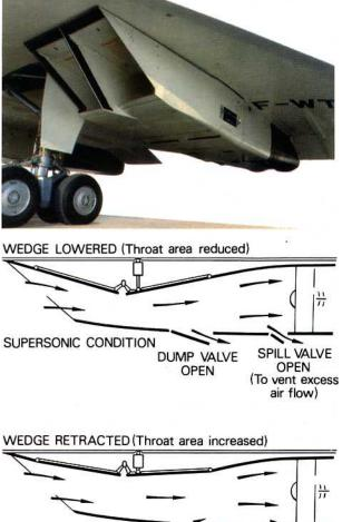
SUBSONIC CONDITION DUMP VALVE (Used as scoop to increase airflow) SPILL VALVE OPEN (To prevent turbulence)
