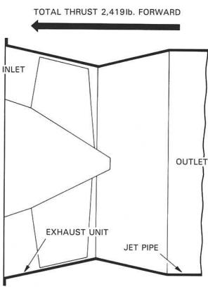
EXHAUST UNIT AND JET PIPE
