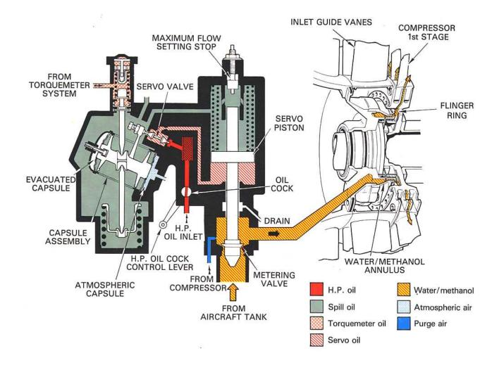
Fig. 17-3 A typical compressor inlet injection system.
