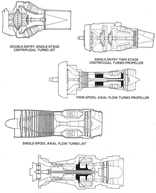
TWIN-SPOOL TURBO-SHAFT (with free-power turbine)
