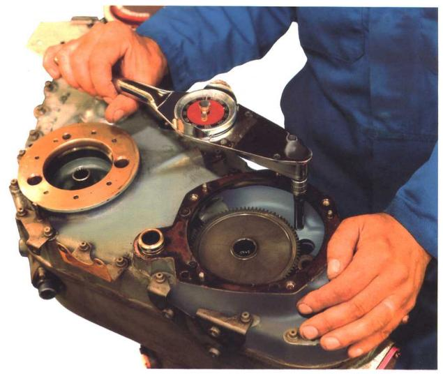
Fig. 25-12 Torque tightening.
