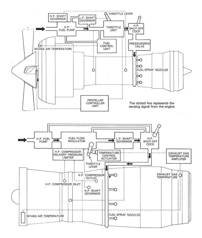
Fig. 10-3 Simplified fuel systems for turbo-propeller and turbo-jet engines.
