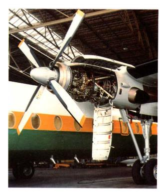
Fig. 23-13 Engine accessibility, turbo-propeller engine.
