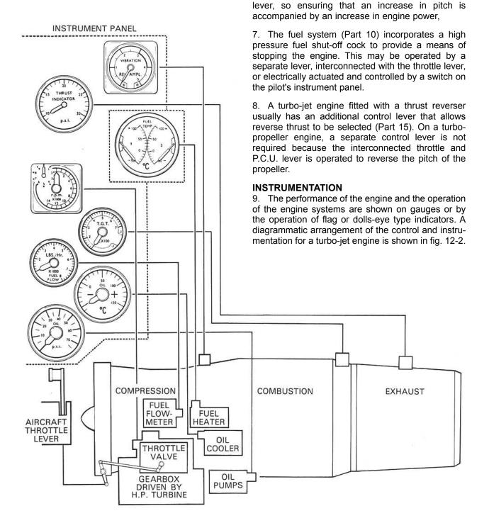
Fig. 12-2 Diagrammatic arrangement of engine control and instrumentation.
