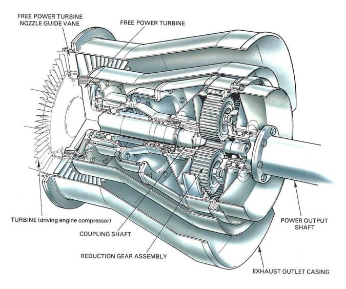
Fig. 5-4 A typical free power turbine.
