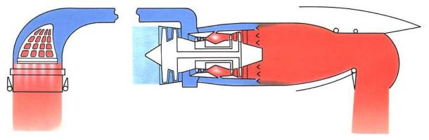
Fig. 18-17 Remote augmented lift system.
