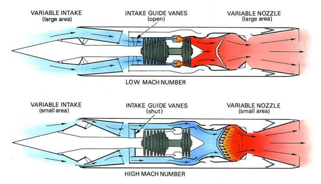
Fig. 1-11 A turbo/ram jet engine.
