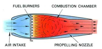
Fig. 1-6 A ram Jet engine.
