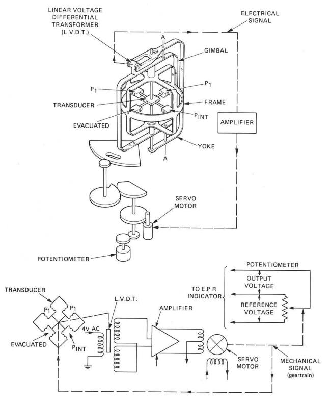
Fig. 12-3 Electro-mechanical E.P.R. transmitter.
