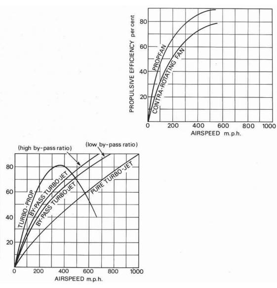
Fig. 21-9 Propulsive efficiencies and aircraft speed.
