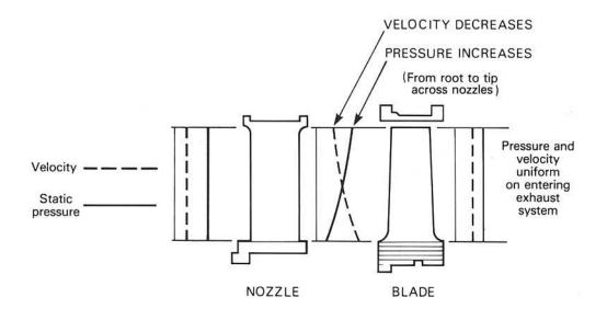
Fig. 5-7 Gas flow pattern through nozzle and blade.
