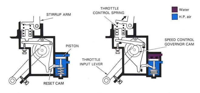
SPEED CONTROL GOVERNOR RESET DEVICE WITH WATER INJECTION NOT SELECTED SPEED CONTROL GOVERNOR RESET DEVICE WITH WATER INJECTION SELECTED
