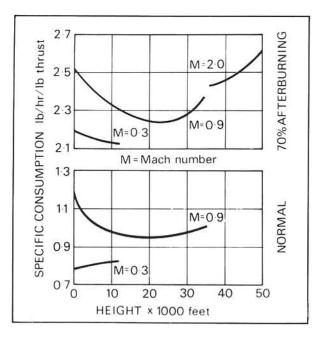
Fig. 16-9 Specific fuel consumption comparison.
