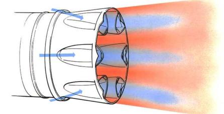
SUPPRESSOR NOZZLE (high mixing rate) REDUCED NOISE LEVEL
