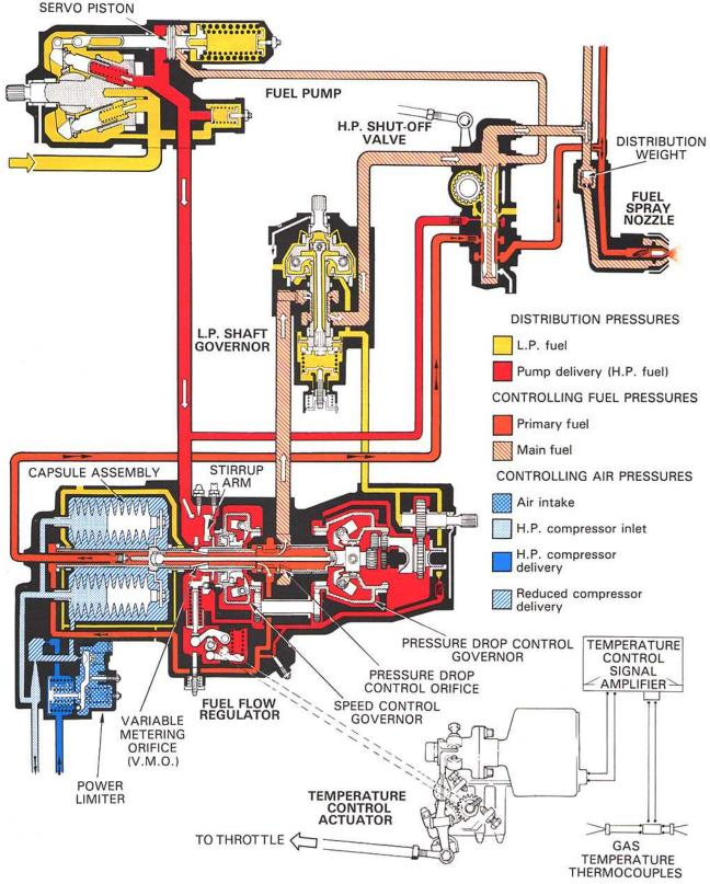
Fig. 10-9 A combined acceleration and speed control system.
