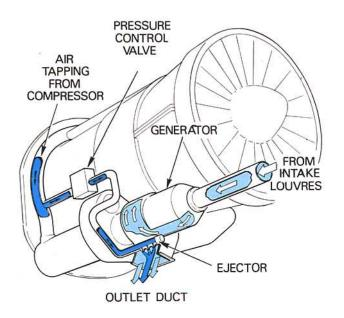
Fig. 9-6 A generator cooling system.
