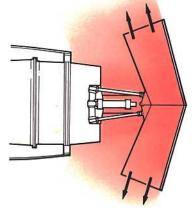
ACTUATOR AND BUCKET DOORS IN REVERSE THRUST POSITION
