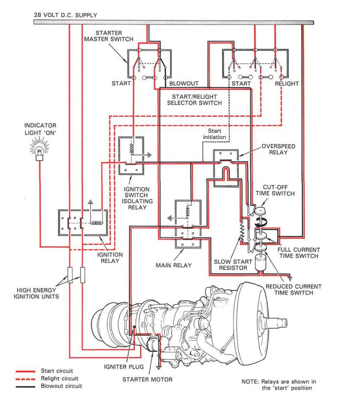
Fig. 11-3 A low voltage electrical starting system.
