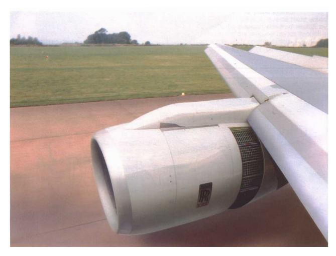
Fig. 15-7 A cold stream thrust reverser installation.
