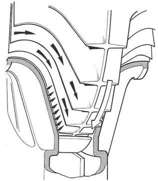
Fig. 3-4 Impeller working clearance and air leakage.
