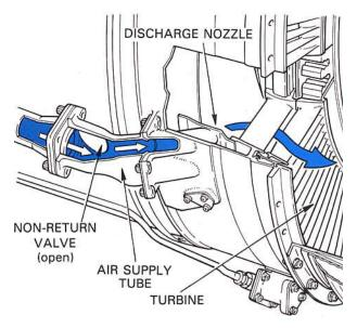
Fig. 11-8 Air impingement starting.
