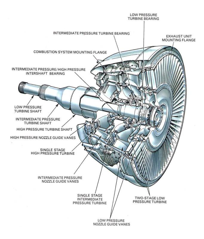
Fig. 5-3 A triple turbine and shaft arrangement.
