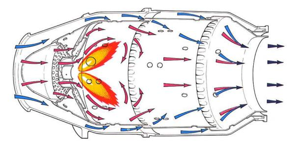
Fig. 4-3 Flame stabilizing and general airflow pattern.
