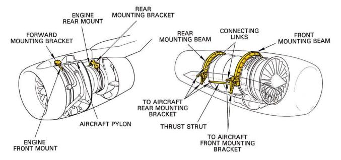
Fig. 23-11 Typical turbo-jet engine mountings.
