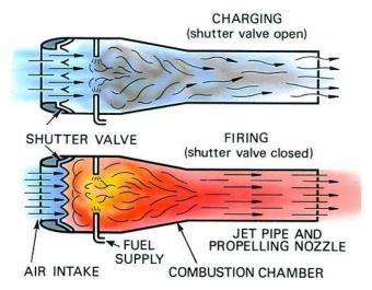
Fig. 1-7 A pulse jet engine.
