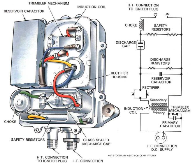
Fig. 11-10 A D.C. trembler-operated ignition unit.
