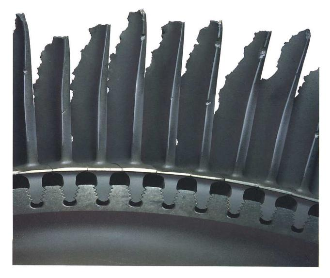
Fig. 24-9 Overheated turbine blades.
