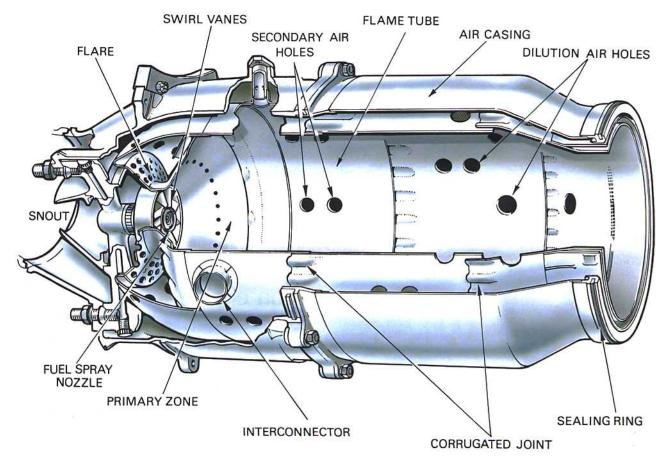
Fig. 4-1 An early combustion chamber.
