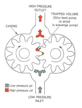
Fig. 8-5 Principle of a gear pump.
