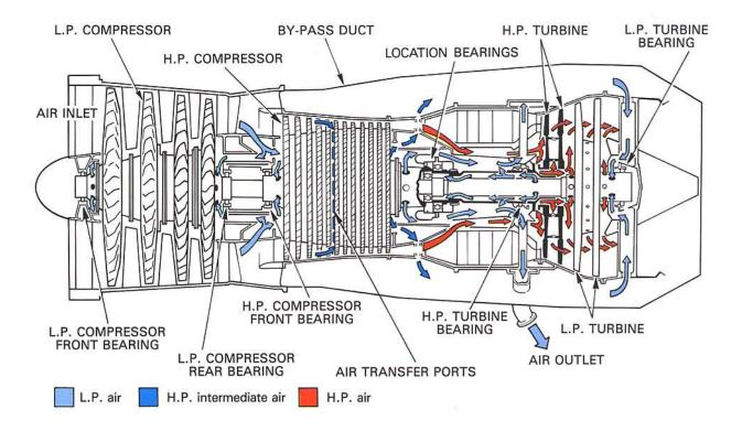
Fig. 9-1 General internal airflow pattern.
