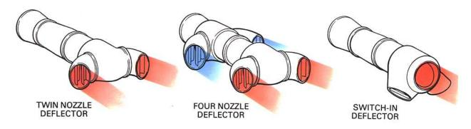
Fig. 18-4 Thrust deflector systems.
