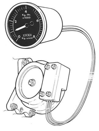
Fig. 12-10 Fuel flow transmitter and indicator.
