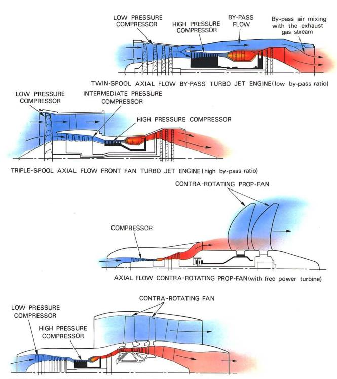
TWIN-SPOOL AXIAL FLOW CONTRA-ROTATING REAR FAN (with free power turbine)
