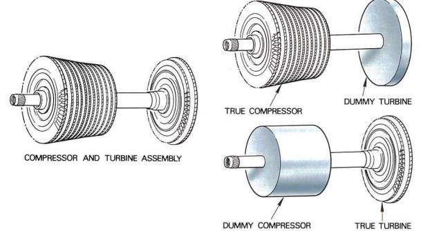
Fig. 25-7 Simulated engine rotor assemblies.
