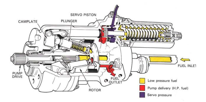
Fig. 10-14 A plunger-type fuel pump.
