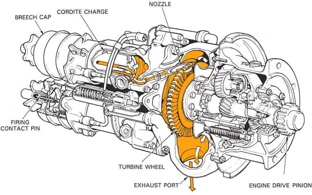
Fig. 11-4 A triple-breech cartridge starter.
