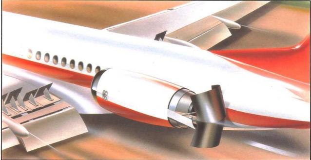
Fig. 15-6 Hot stream thrust reverser installations.
