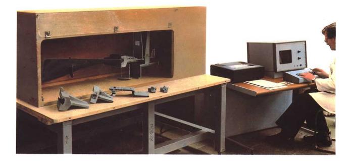
Fig. 25-8 Principle of blade moment weighing.
