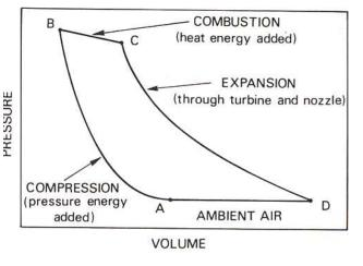
Fig. 2-2 The working cycle on a pressure-volume diagram.
