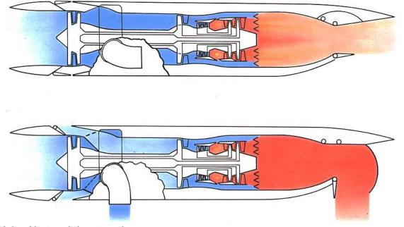
Fig. 18-9 Vectored thrust engine.
