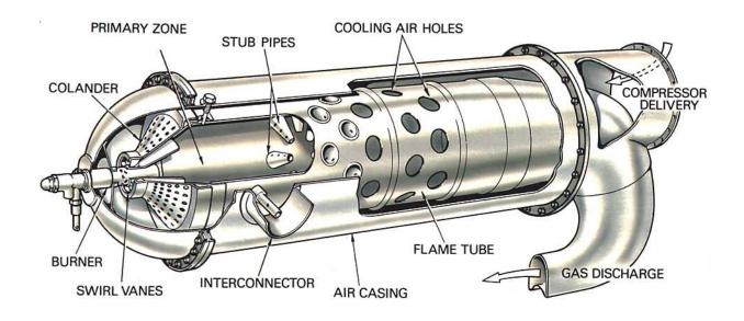
Fig. 4-6 An early Whittle combustion chamber.
