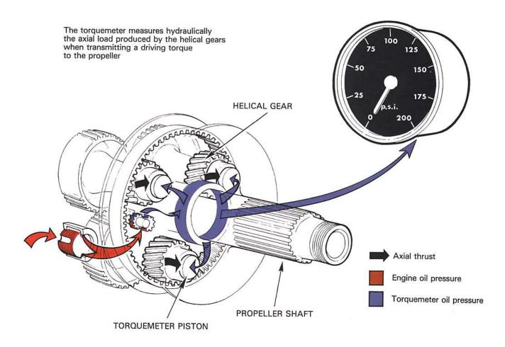
Fig. 12-4 A simple torquemeter system.
