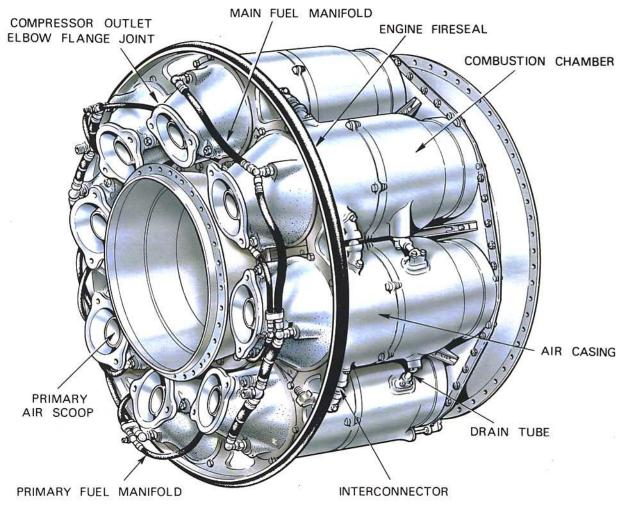
Fig. 4-7 Multiple combustion chambers.
