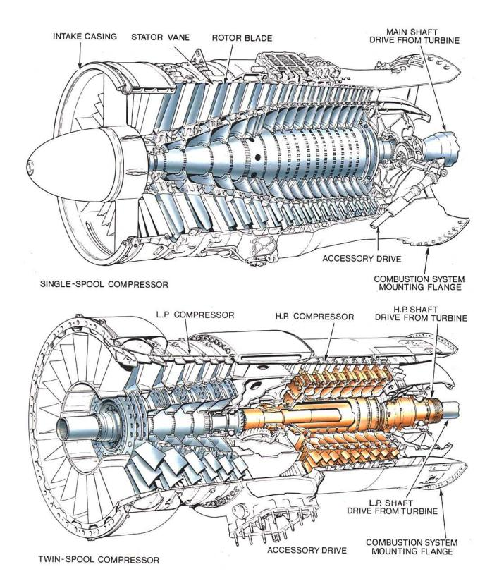
Fig. 3-7 Typical axial flow compressors.
