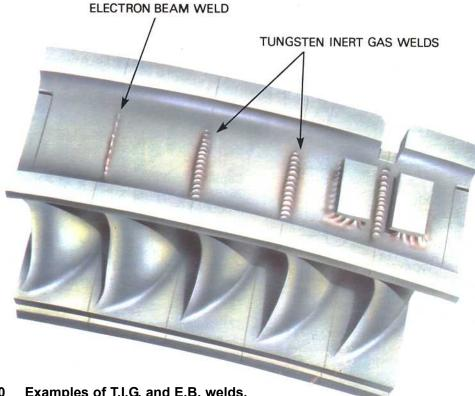
Examples of T.I.G. and E.B. welds. Fig. 22-10
