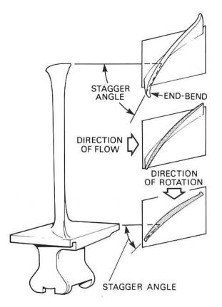
Fig. 3-12 A typical rotor blade showing twisted contour.
