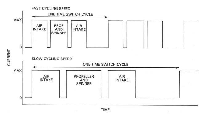
Fig. 13-5 Typical ice protection cyclic sequence.
