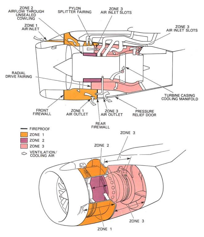
Fig. 14-2 Cooling and ventilation - turbo-fan engine.
