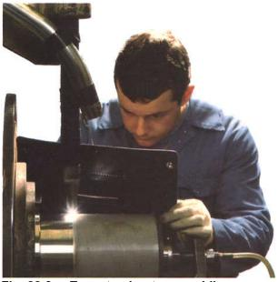
Fig. 22-8 Tungsten inert gas welding.
