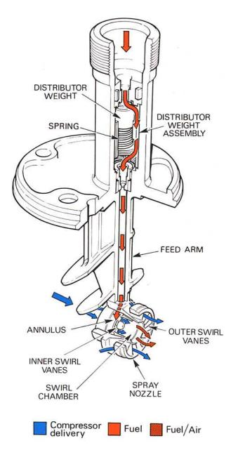
Fig. 10-19 An airspray nozzle.
