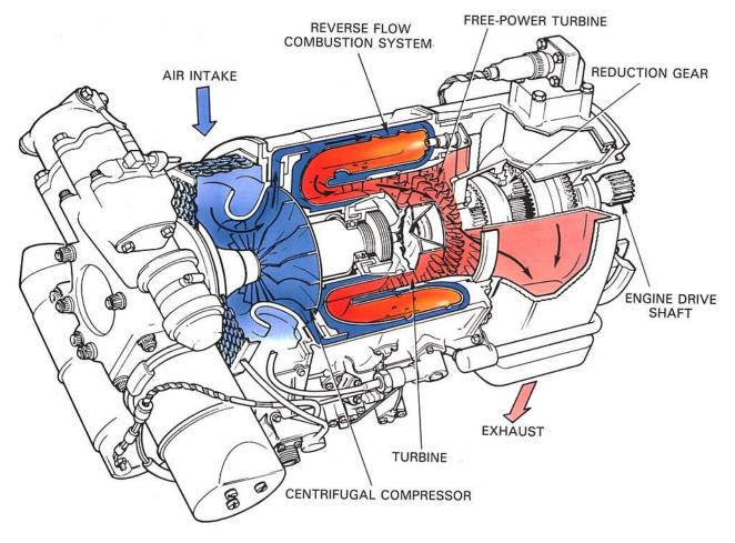
Fig. 11-9 A gas turbine starter.
