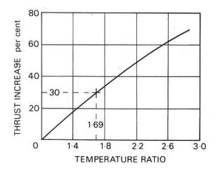
Fig. 16-8 Thrust increase and temperature ratio.
