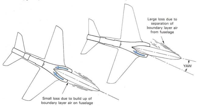
Fig. 23-7 Loss of ram pressure in divided intakes.
