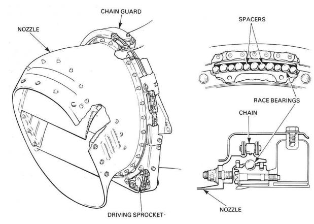
Fig. 18-6 Side mounted swivelling nozzle.
