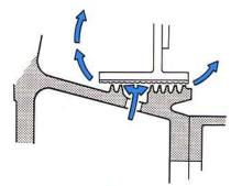
CONTINUOUS GROOVE INTERSTAGE (labyrinth) AIR SEAL
