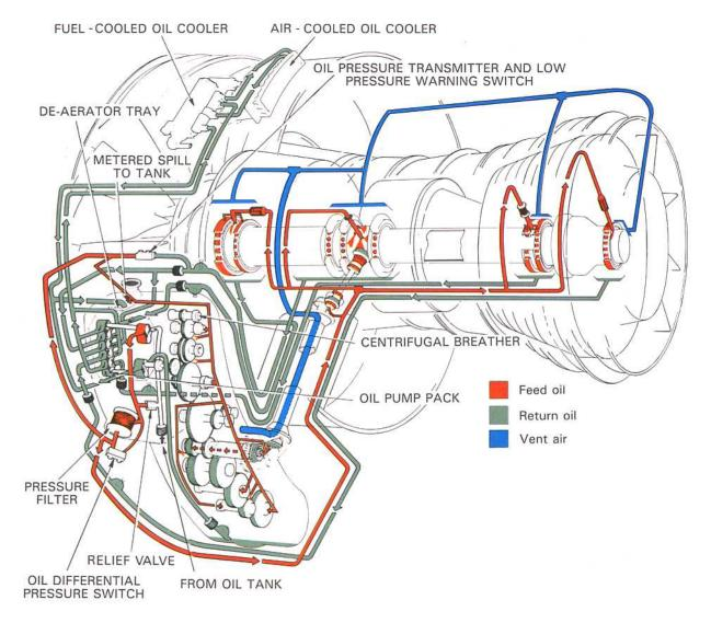
Fig. 8-2 A full flow type oil system.
