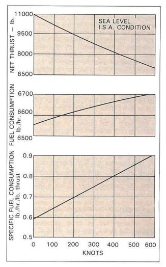
Fig. 21-4 The effect of aircraft speed on thrust and fuel consumption.
