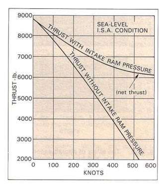
Fig. 21-3 Thrust recovery with aircraft speed.
