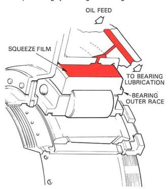
Fig. 8-9 A squeeze film bearing.
