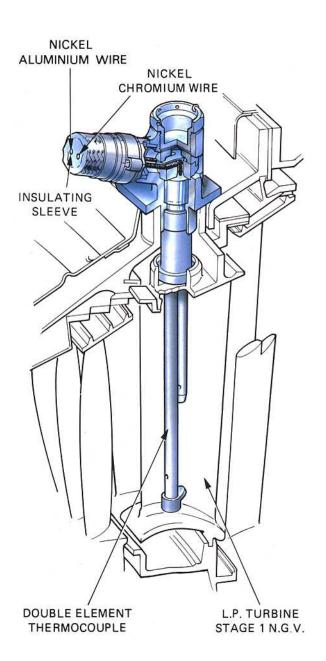
Fig. 12-7 Turbine thermocouple installation.
