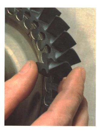
Fig. 5-14 Ceramic turbine blades.
