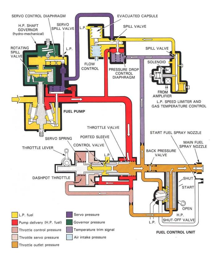
Fig. 10-5 A pressure control system (turbo-jet engine).
