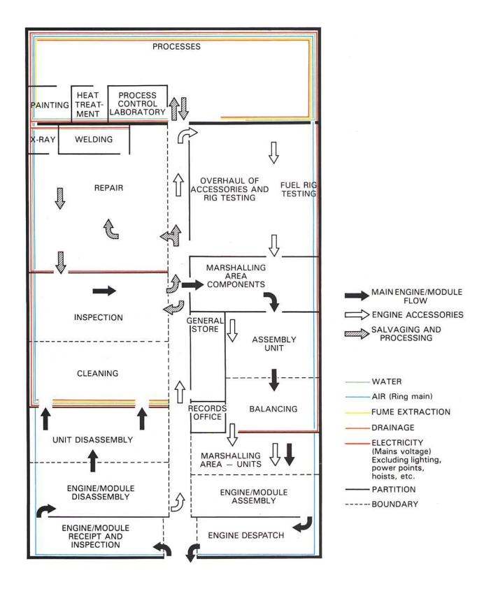
Fig. 25-2 Typical overhaul workshop layout.
