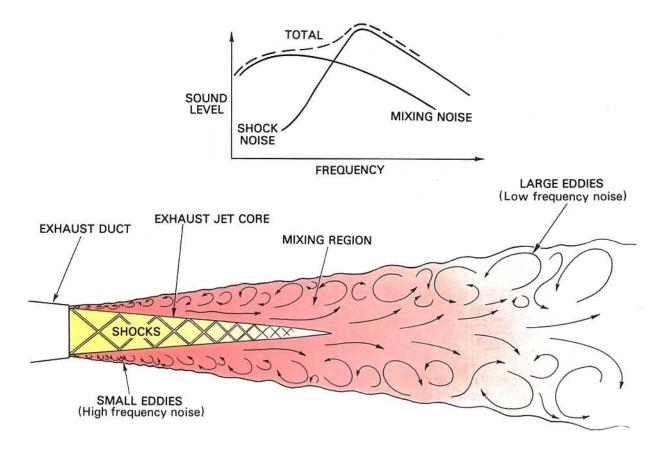
Fig. 19-2 Exhaust mixing and shock structure.
