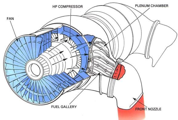
Fig. 18-16 Plenum chamber burning.
