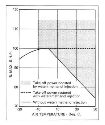
Fig. 17-2 Turbo-propeller power boost.
