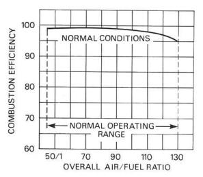
Fig. 4-10 Combustion efficiency and air/fuel ratio.
