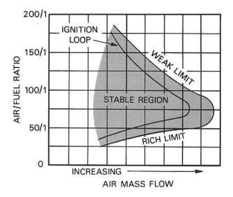
Fig. 4-11 Combustion stability limits.
