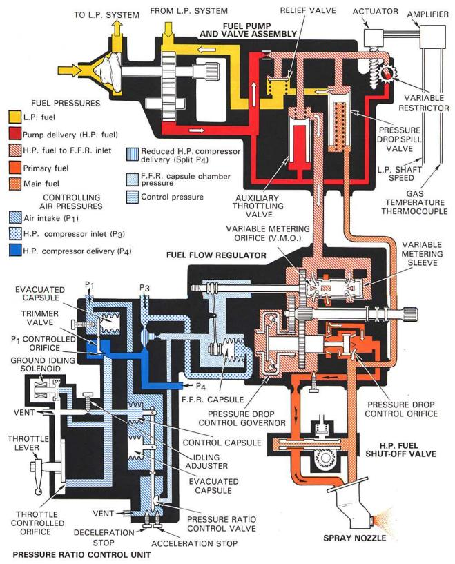
Fig. 10-12 A pressure ratio control system.
