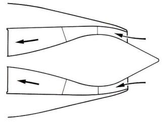
Fig. 23-8 External/internal compression intake.
