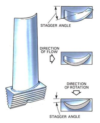
Fig. 5-6 A typical turbine blade showing twisted contour.
