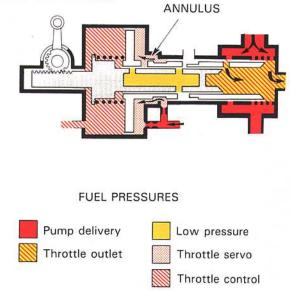
Fig. 10-6 Acceleration control by dashpot throttle.
