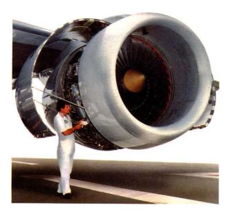
Fig. 23-12 Engine accessibility, turbo-fan engine.
