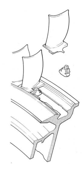
Fig. 3-11 Methods of securing blades to disc.
