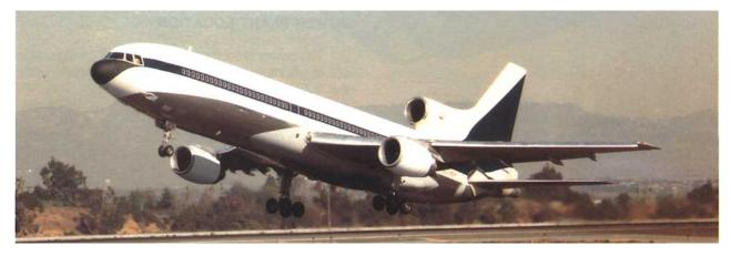
Fig. 23-3 Tail and wing-mounted pod installation.
