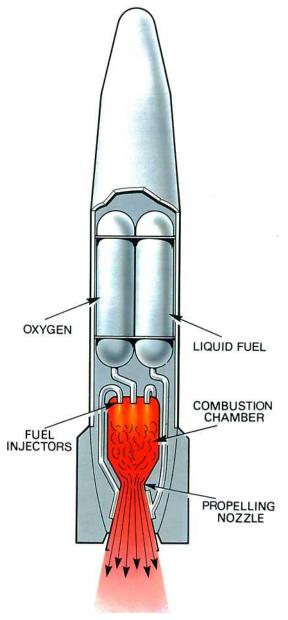
Fig. 1-8 A rocket engine.
