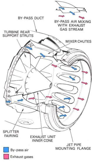
Fig. 6-4 A low by-pass air mixer unit.
