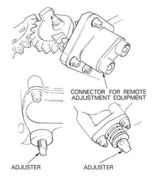
Fig. 24-5 Typical friction locked adjusters.
