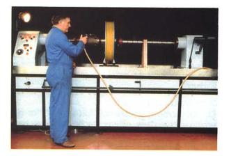
Fig. 25-3 Magnetic crack testing.
