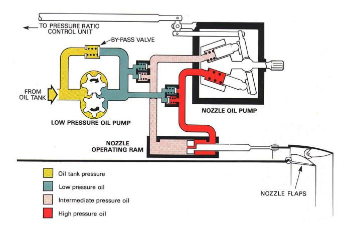
Fig. 16-7 A simplified typical afterburner nozzle control system.
