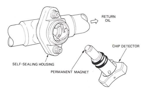
Fig. 8-8 A magnetic chip detector.
