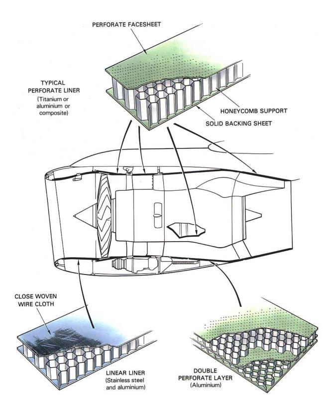
Fig. 19-6 Noise absorbing materials and location.
