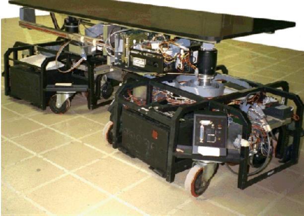
**Figure 2:** The experimental dual differential drive vehicle, built and tested at the University of Michigan.
