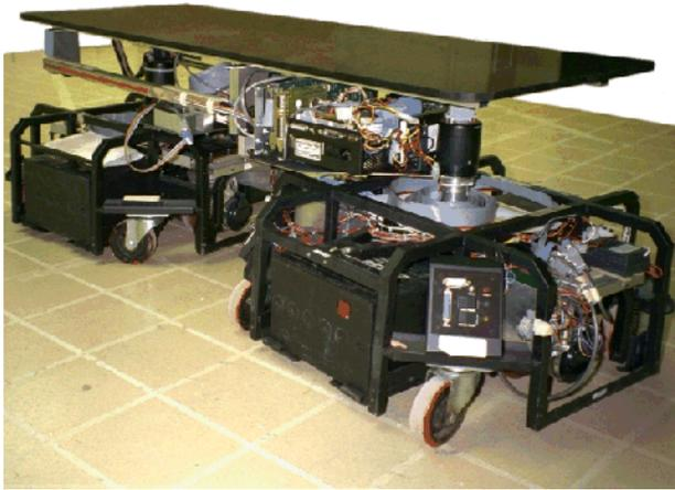
**Figure 2:** The experimental dual differential drive vehicle, built and tested at the University of Michigan.
