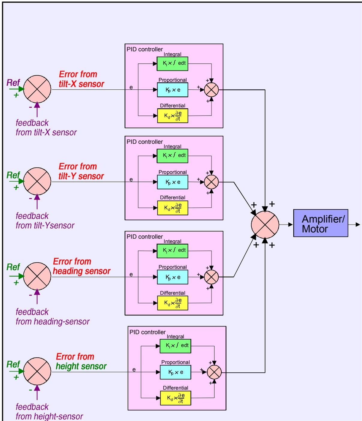
Figure 7: Additive control system in the experimental prototype. Four different feedback signals are fed into each actuator. The Hoverbot has eight actuators.
