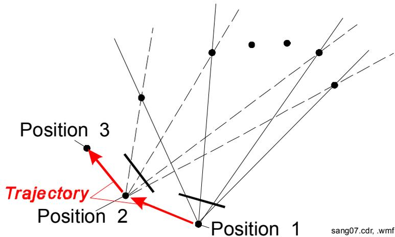
Figure 9.7: Illustration of map building and trajectory integration.
