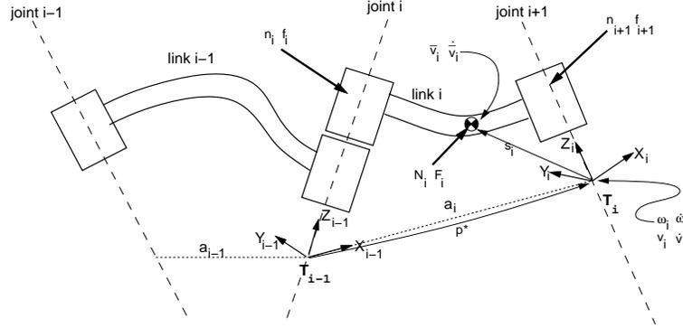
Figure 2: Notation used for inverse dynamics, based on standard Denavit-Hartenberg notation.
