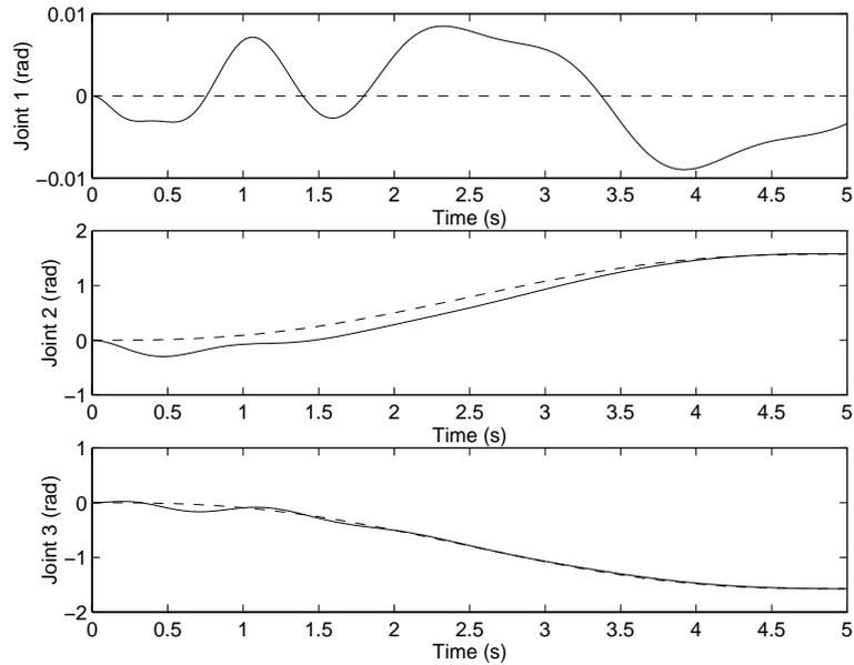
Results of `fdyn()` example. Simulated path shown as solid, and reference path as dashed.
