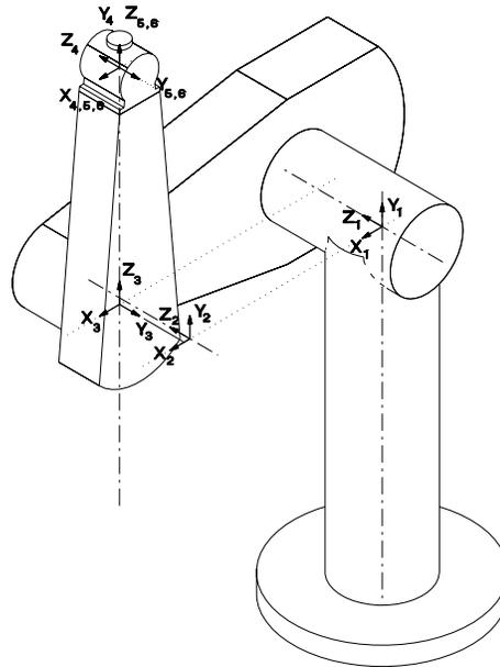
Details of coordinate frames used for the Puma 560 shown here in its zero angle pose.
