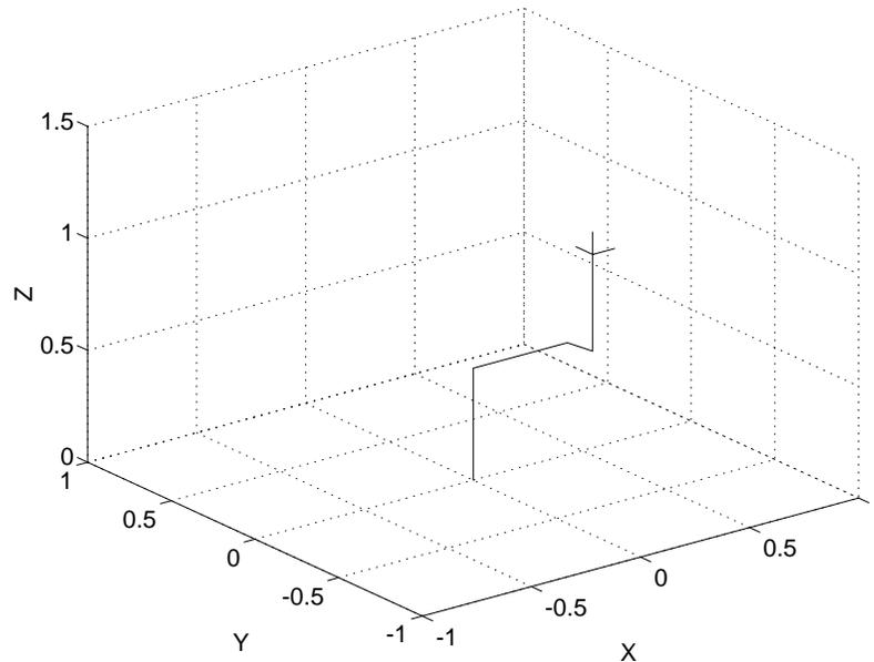
The wrist coordinate frame is shown by 3 short orthogonal line segments which are colored: red (X or normal), green (Y or orientation) and blue (Z or approach).
