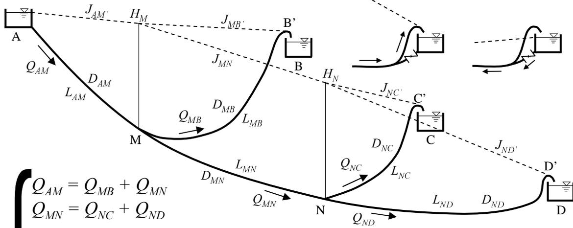
$$\left\{ \begin{array}{l} Q_{AM} = Q_{MB} + Q_{MN} \\ Q_{MN} = Q_{NC} + Q_{ND} \\ Z_A - H_M = J_{AM} \cdot L_{AM} \\ H_M - Z_{B'} = J_{MB'} \cdot L_{MB} \\ H_M - H_N = J_{MN'} \cdot L_{MN} \\ H_N - Z_{C'} = J_{NC'} \cdot L_{NC} \\ H_N - Z_{D'} = J_{ND'} \cdot L_{ND} \end{array} \right.$$
