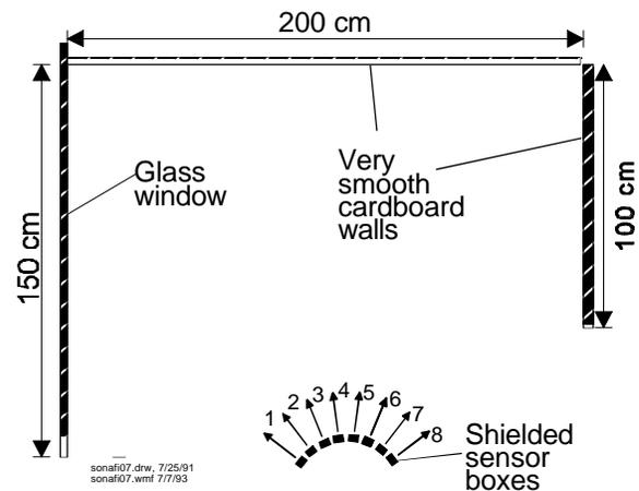
**Figure 4:** Experimental set-up in crosstalk-promoting environment.
