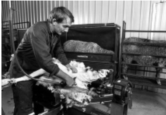
Figure 6. SLAMP manipulator simplified and refined for manual shearing (1996).
