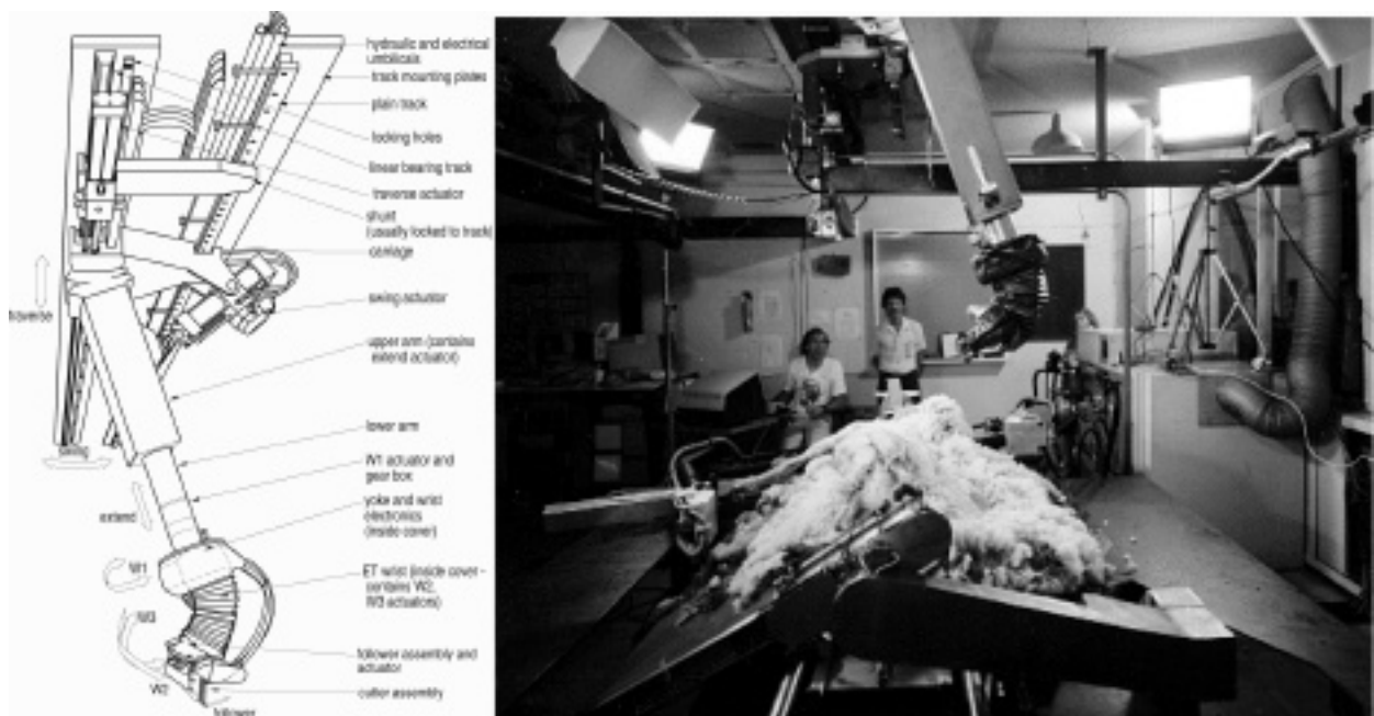
Figure 4. SM Robot and SLAMP manipulator. Photograph shows a shearing demonstration in 1989.
