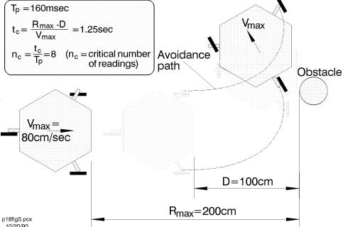
Figure 5: With a maximum range of  $R_{\text{max}}$ =200cm and a minimal avoidance growth rate operator(GRO) distance D=100 cm, CARMEL has 1.28 sec to produce an obstacle cluster to increment a cell (i,j) faster strength (OCS) strong enough to cause an avoidance maneuver. when the immediate neighbors of the cell hold high CVs. This function is implemented in real-time by convolving  $CV_{i,j}$  with the  $3\times3$  mask given in Fig. 6b, and adding the usual increment  $I^+$ =3, yielding
