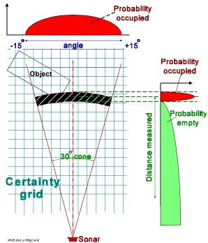
**Figure 2:** Two-dimensional projection of the conical field of view of an ultrasonic sensor. A range reading *d* indicates the existence of an object somewhere within the shaded region A (Carnegie Mellon's model).
