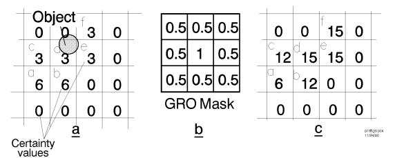
**Figure 6:** a. In-motion sampling causes sonar readings of an object to be scattered over several cells, resulting in a low OCS.
